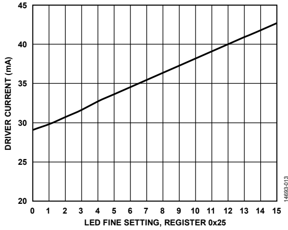
Figure 16. LED Driver Current vs. LED Fine Setting (Coarse Setting = 0x0)
