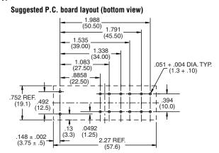
27E1081 - 6 pole socket for use with SCHRACK SR6 series relay, types with 5NO + 1NC contacts
