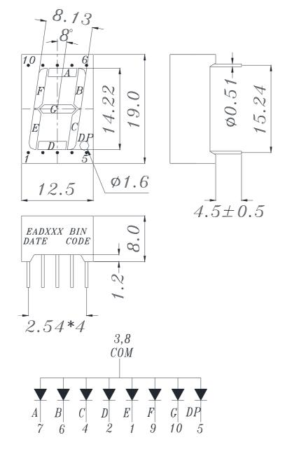
Note: Tolerances unless mentioned ±0.25mm. Unit = mm
