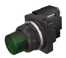
30mm BlackMax, Epoxy Coated Corrosion Resistant Complete Metal Unit Illuminated Indicator Light Transformer type, 240V AC Incandescent Lamp, BA9s Glass Lens, Green UL Listed, CSA Certified NEMA 1,3,3R,4,4X,12,13 & Automotive Standards
