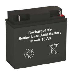
General Series Valve Regulated Lead Acid batteries are designed with AGM (Absorbent Glass Mat) technology, high performance plates and electrolyte to gain extra power output for many commonly used applications. Special one-way valves allow excessive gases to escape but otherwise the battery is completely sealed and therefore maintenance-free, leak proof and usable in any position
