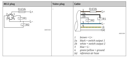
*IO-Link: 2 x PNP switch output R1 and R2*
