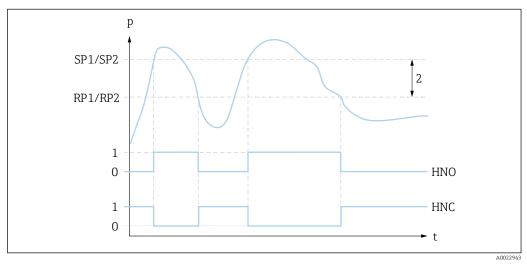
■ 1 SP1/SP2: switch point 1/2; RP1/RP2: switch-back point 1/2
