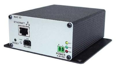
The EM1500 Serial-Ethernet Bridge is a device that converts multi-point serial communications to a TCP/IP network. The EM1500 connects to and network enables as many as 4 RS-232 serial devices simultaneously. In addition, the EM1500 provides an SPDT relay, 2 digital open collector outputs and 3 digital inputs suitable for interfacing to mechanical switches or logic level circuits.
