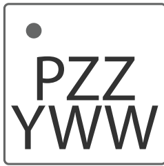
Figure 15 ■ Package Marking Specifications for PE42424
