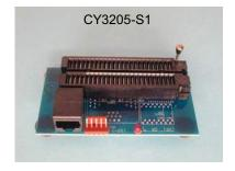
To accommodate the largest number of pin counts with each board, the largest socket is installed. For example, the CY3205-S1 includes a 48-pin DIP socket. It therefore supports 8, 20, 28, and 48-pin DIP parts. The CY3205-S3 includes a 28-pin SSOP socket that can accept both the 20 and 28-pin SSOP parts. The body width of the 48-pin SSOP package is wider than the 20 and 28-pin so the CY3205-S4 is necessary for the 48-pin SSOP parts.
