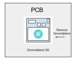
In all cases, the requirement to run traces under the module may arise. This is allowed provided there are no traces run through the RF KEEPOUT area described in the Recommended Pad Layout section above. Beware that high speed data lines running under the module is not recommended as there might be interference in both directions (host to module and module to host) especially when the module executes a transmission.
