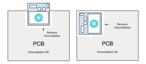
Based on the above recommendations, there may be situations where you cannot place the module near an edge. This may force the module to buried within the center groundplane of the host base board. Even though this is not recommended due to the dramatic decrease in chip antenna performance, the U.FL connections will still provide adequate RF performance to the external antenna of choice. As long as the ground plane can be minimized under the module as shown in the following figure.
