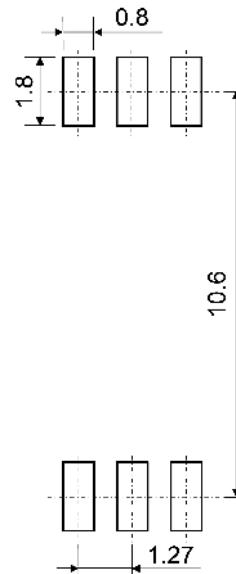
Fig. 15.2 Lead forming and taping option (LF4), (TP4)
