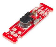
The FemtoBuck is a small-size, single-output constant current LED driver. By default, the FemtoBuck is driven at 350mA. That current can be reduced by either presenting an analog voltage or a PWM signal to the board.
