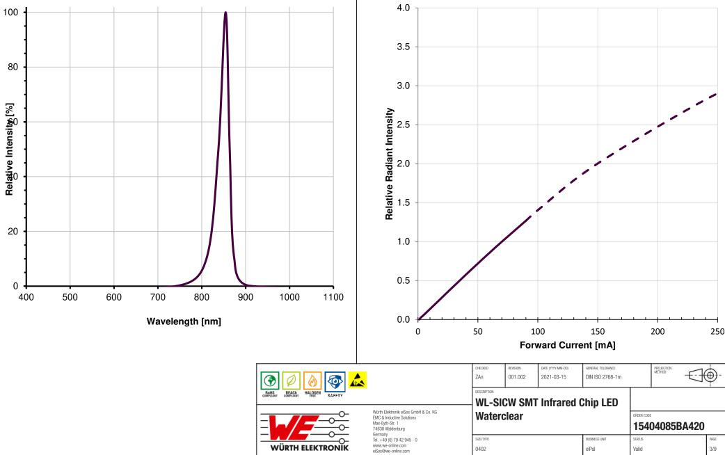
**Relative Radiant Intensity vs. Forward Current:**
