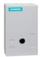
Non-reversing NEMA contactor, Size 1, Three phase full voltage, Contactor amp rating 27A, 3 wire (NO aux included), 380-440/440-480V 50/60Hz coil, Non-combination type, Enclosure NEMA type 1, Indoor general purpose use, Standard width enclosure
