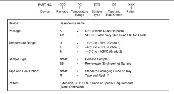
Note 1: Tape and Reel identifier only appears in the catalog part number description. This identifier is used for ordering purposes and is not printed on the device package. See "Orderable Part Numbers" below or check with your Microchip Sales Office for package availability with the Tape and Reel option.
