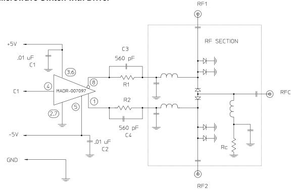
Selection of PIN diodes and bias structure values will affect the switching speed. For switching speed applications slower than 1  $\mu$ s, remove C3, C4 and RC.
