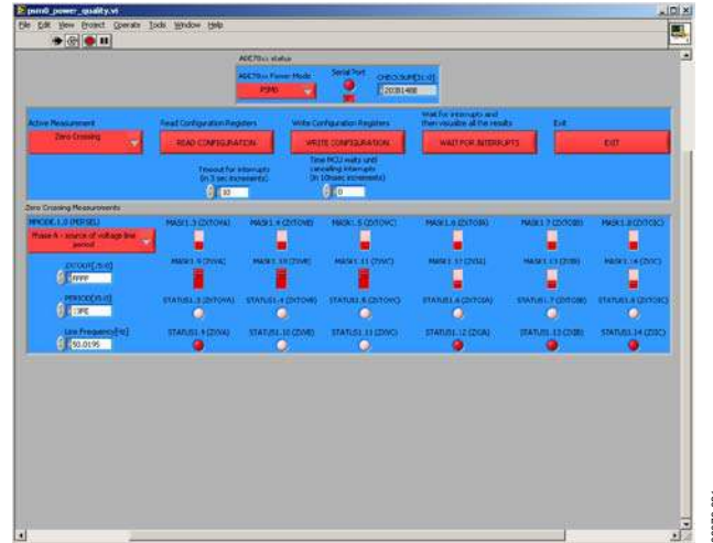
Figure 21. Power Quality Zero-Crossing Measurements Panel
