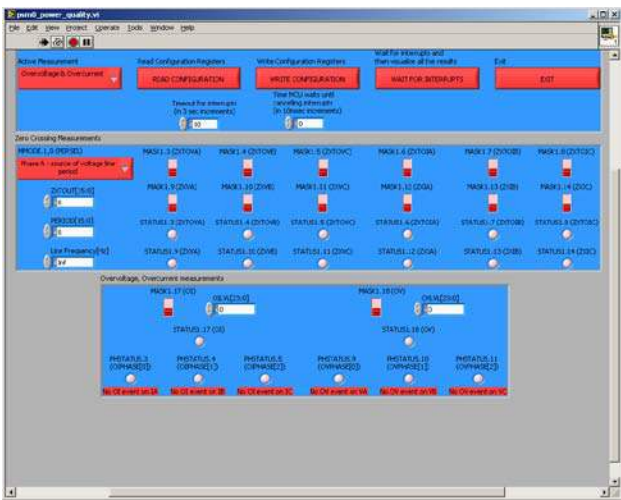
Figure 23. Overvoltage and Overcurrent Measurements Panel
