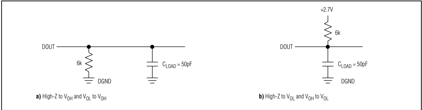
Figure 1. Load Circuits for DOUT Enable Time
