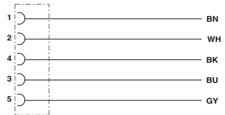
Contact assignment of the M12 socket
