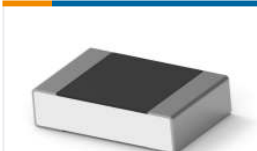
TE Part #3-2176381-2 RQ 0805 26K1 0.1% 10PPM 5K RL
