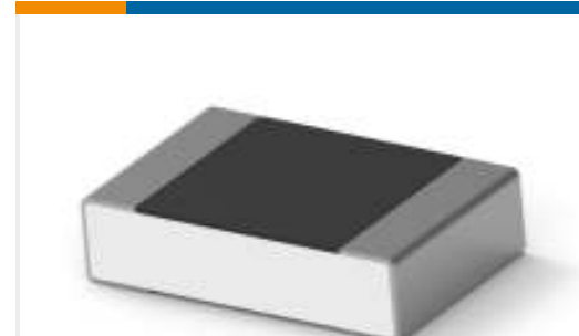
TE Part #4-2176381-6 RQ 0805 36K5 0.1% 10PPM 5K RL
