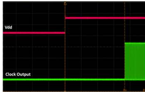
Figure 17. Startup Waveform vs. Vdd
