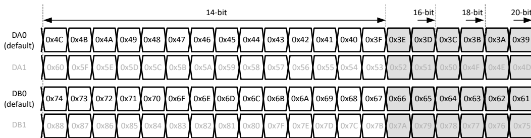
Figure 8-38. 1-wire output bit mapping
