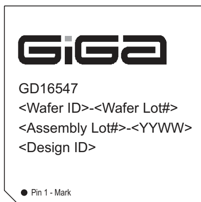
Figure 8. Device Marking, Top View
