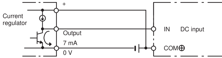
NPN open-collector output
