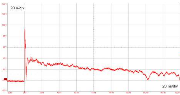
Figure 4. ESD response to ISO 10605 - C = 150 pF, R = 330 \Omega (+8 kV contact discharge)
