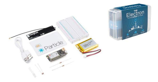
**Description:** The Electron is a tiny development kit for creating 3G cellular-connected electronics projects and products. It comes with a Particle SIM card (Nano 4FF) and an affordable data plan for low-bandwidth applications. Plus, it's available to more than 100 countries worldwide, and includes three months of Particle's 1MB monthly data plan for IoT devices!
