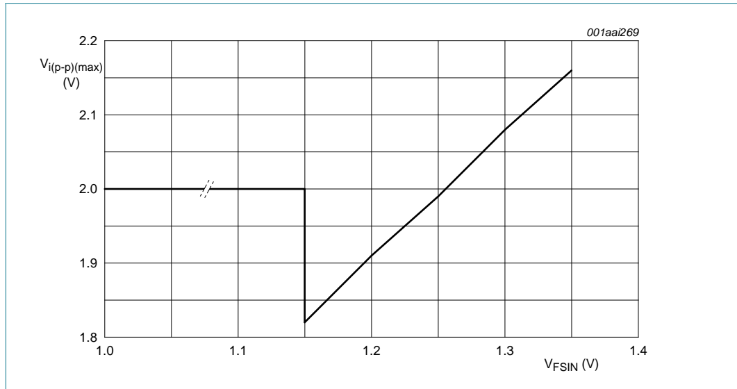
Fig 8. ADC maximum peak-to-peak input voltage V_{i(p-p)(max)} as a function of V_{FSIN}
