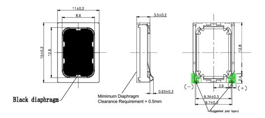
General tolerance = ±0.2 mm and all measurements in mm unless otherwise noted.
