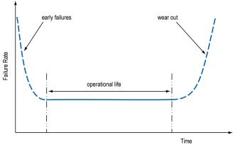
The failure rate is derived from our periodic test results. The failure rate  $(\lambda_R)$  is, therefore, only given at test temperature for life tests. An estimation is also given at 60°C. The expected failure rate for this capacitor range is based on our periodic test results for capacitors with structural similarity.
