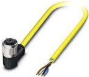
Sensor/Actuator cable, 4-position, TPE, yellow RAL 1021, free cable end, on Socket angled M12 SPEEDCON, A-coded, Cable length: 5 m
