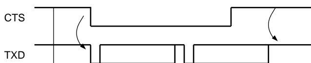
Figure 30-19. Transmitter Behavior when Operating with Hardware Handshaking
