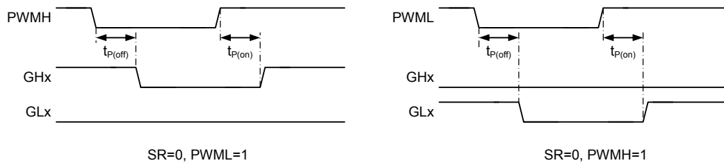
Gate Drive Timing – PWM inputs, Slow Decay, Diode Rectification
