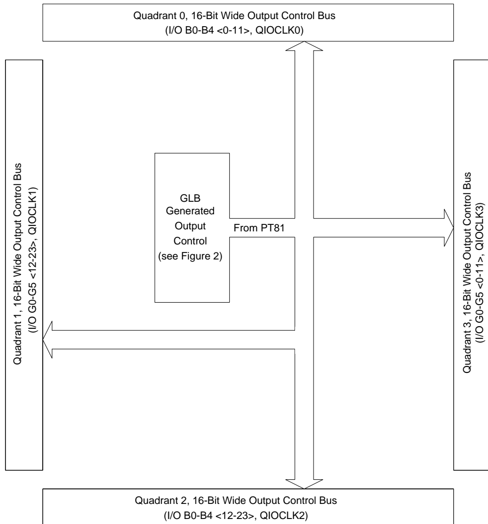
Figure 5. Output Control Bus and Quadrant Organization
