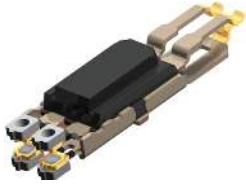
Unique, patent-pending triad wafer design (individual triad close-up)
