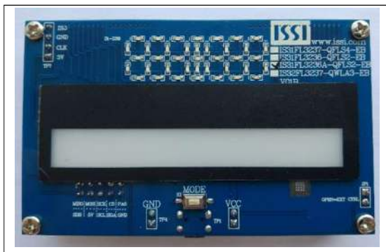
Figure 1: Photo of IS31FL3236A Evaluation Board (Please refer to Appendix I if MCU is LPC922)
