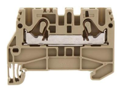
Feed-through installation terminal, Push-in connection, Mounting type: Mounting rail TS 35/7.5, Rated cross-section: 4 mm², Width: 5.1 mm, Colour: Beige
