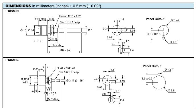
(1) CAUTION: Ø 1.5 of panel cut out must not be fully through-hole
