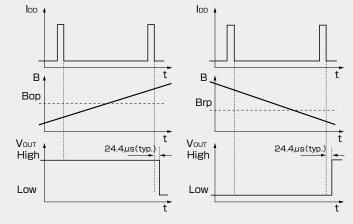
Operating Point Timing Releasing Point Timing This Hall effect IC's output is held as internal data just before the internal circuit 36
