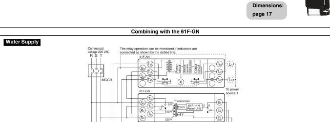
Note: Be sure to ground the common Electrode E<sub>3</sub> (the longest Electrode).
