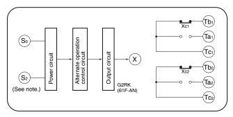
$\left( \begin{array}{c} \text{Note:} \text{ The above diagram is for a rated voltage of 200 or 220 VAC.} \\ \text{Power is supplied to $S_0$ and $S_1$ for 100 or 110 VAC.} \end{array} \right.$
