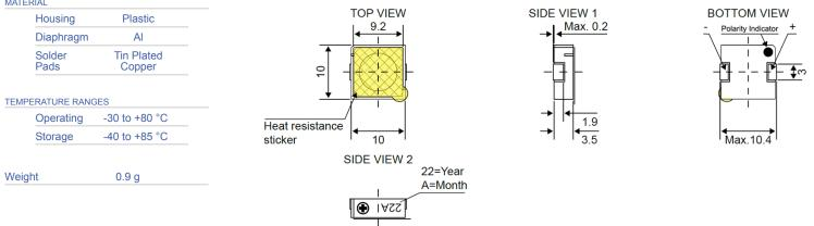
All measurements are mm and general tolerance are ±0.5 unless noted otherwise.
