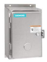
Non-reversing contactor, Size 1P, Single phase full voltage, Contactor amp rating 35A, 3 wire (NO aux included), 24VAC 50-60Hz coil, Non-combination type, Encl NEMA type 4X 304 S-Steel, Water/dust tight noncorrosive, Standard width enclosure
