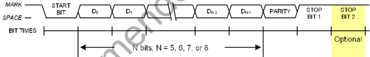
Figure 26.3. UART1 Timing With Parity
