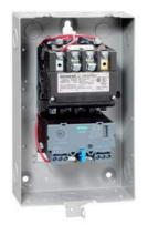
Non-reversing motor starter Size 1 Three phase full voltage Solid-state overload relay OLRelay amp range 0.25-1A 240VAC 50HZ / 277VAC 60HZ coil Combination type Indoor general purpose use
