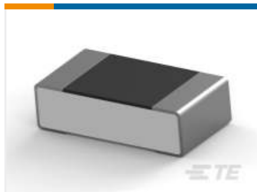
TE Part #9-2176370-7 RQ 0603 4K32 0.1% 10PPM 5K RL
