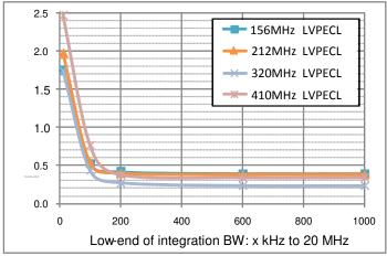
LVPECL Phase jitter (integrated phase noise)
