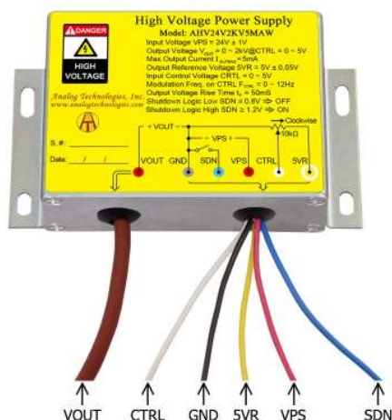
Figure 2. The Connecting Lead Wires of AHV24V2KV5MAW
