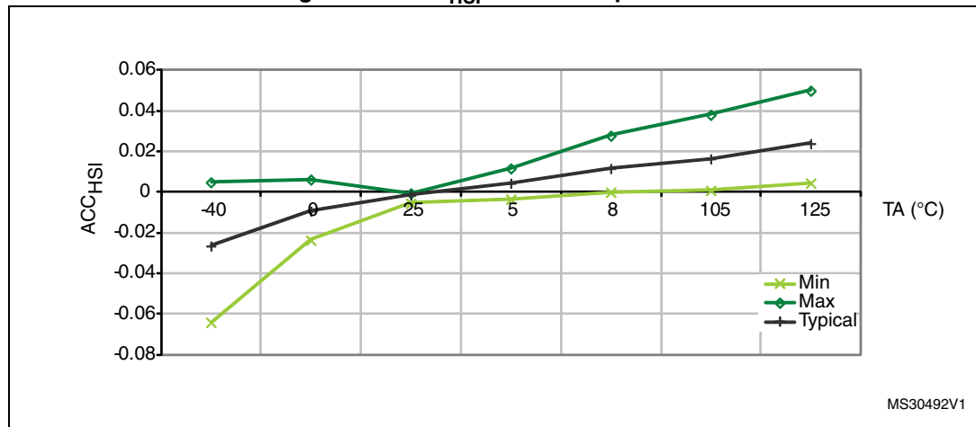
Figure 23. ACC_{HSI} versus temperature
