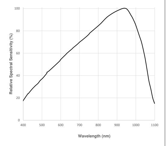
Testcondition:  $Ee = 0.5 \text{ mW/ cm}^2$ , VCE = 5 V
