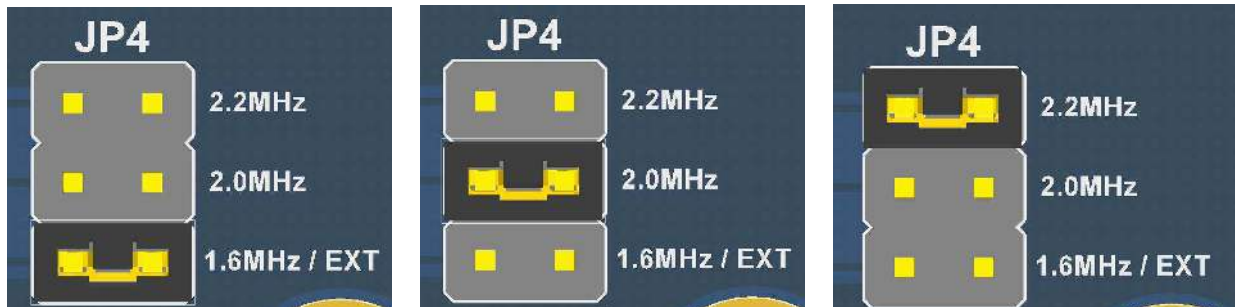
Figure 2. RT Jumper Settings
