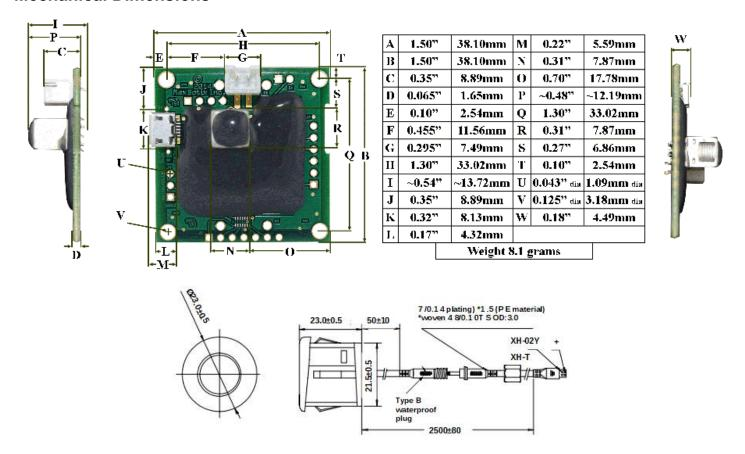
**Note:** Dimension for "K" and "W" are not applicable on MB8460/MB8480 CarSonar-WR sensors. The recommended operating and storage temperature of the CarSonar-WR is -40C to +75C.
